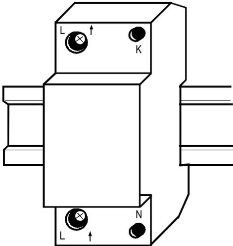
The connection diagram shows how to install the DIN 63 A FD 10 filter coupler correctly: behind the residual current circuit breaker, yet in front of the fuses for separate circuits. The filter is mounted by simply snapping it onto the DIN rail (see figure) and has the following screw-type terminals:
