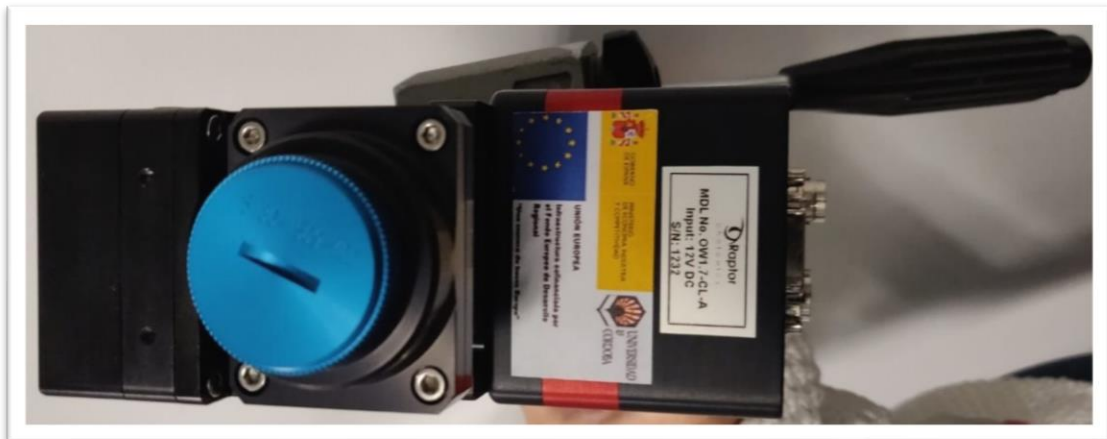
Figura 1. Cámara Hyperespectral Headwall Photonics Micro-Hyperspec NIR R320
